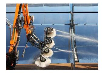
Vehicle for cleaning the parabolic troughs.
