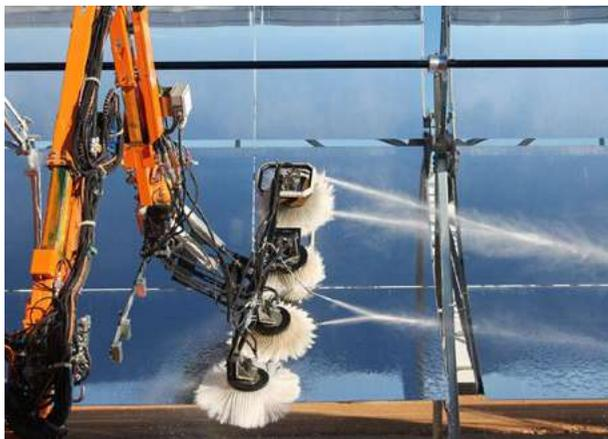
Vehicle for cleaning the parabolic troughs.
