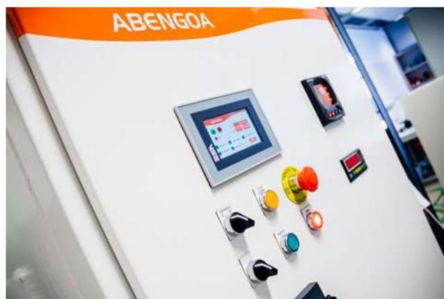
100 MW electric motor converter.
