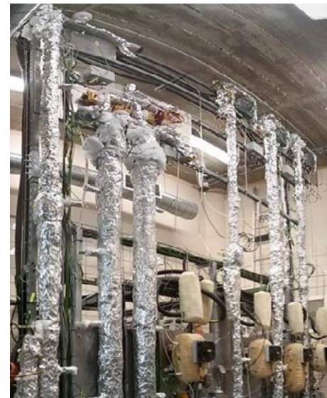
Pilot unit to separate and purify butanol
