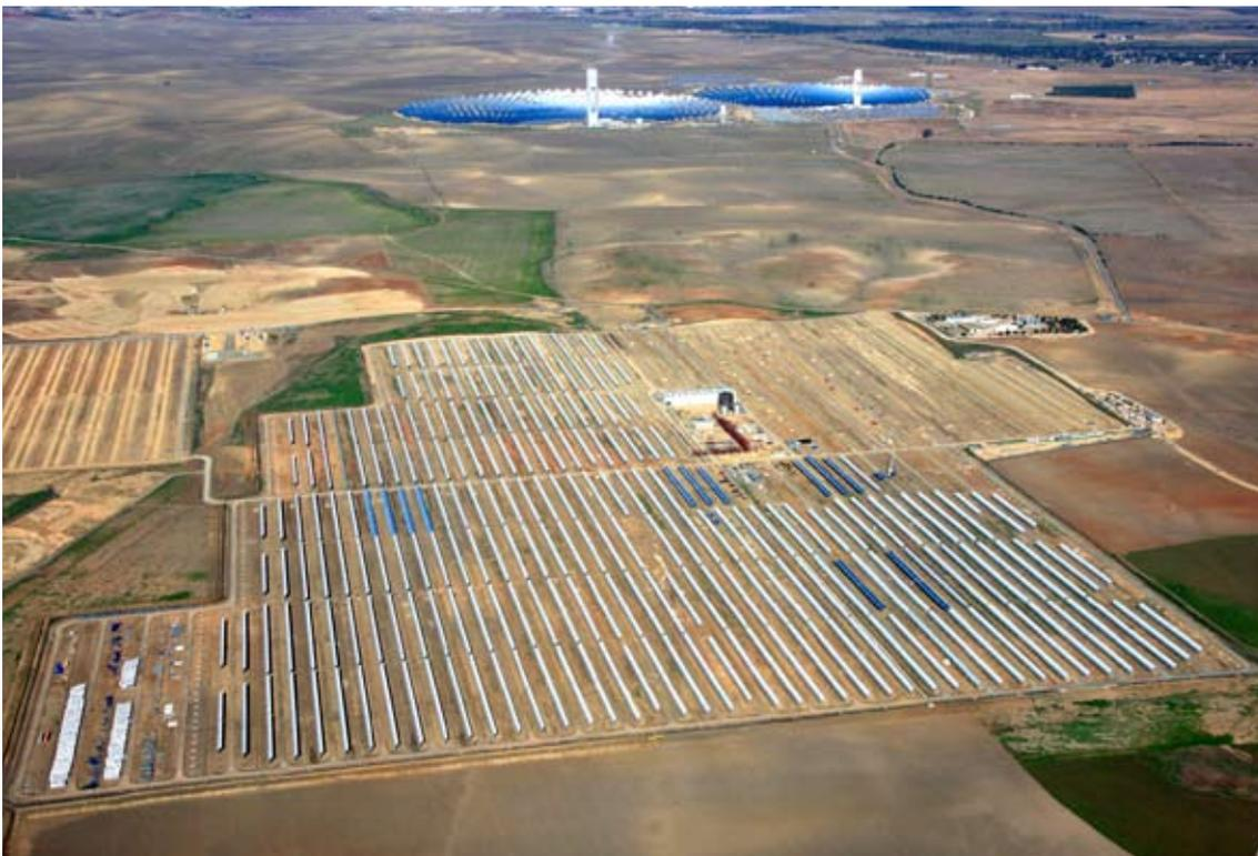
The technology consists of concentrating solar radiation by means of high-precision curved mirrors onto a heat-absorbing pipe, inside which circulates a fluid that reaches high temperatures. This fluid enables the production of steam that is sent on to a turbo-generator, where it expands in order to produce energy.
